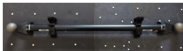
Fig. 1 The pattern for testing scanners' precision.
