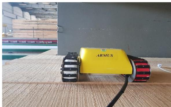
*Fig. 11 a Second generation ARMUS robot - front view*
