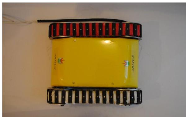
*Fig. 11 a Second generation ARMUS robot designed to work both underwater and on "dry" iron surface - top view*
