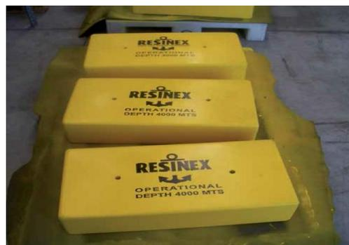
Fig. 2 Resinex syntactic foam blocks
