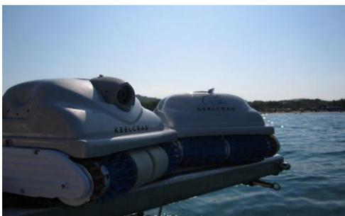
*Fig. 9 Keelcrab hull cleaning robot*
