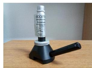
**Fig. 4** 50x magnification microscope
