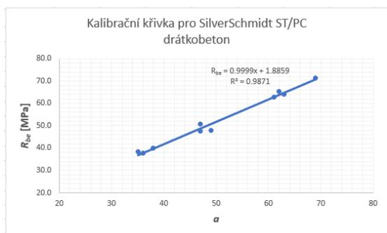
**Fig. 1** Calibration curve for Silverschmidt ST / PC
