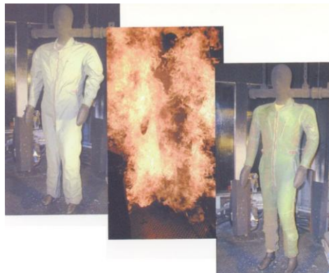
Fig.1 Mannequins dressed with "Nomex" for test in a camera
