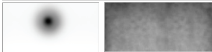
Fig.6. Images of Russian anti-tank mines TM-62M (metal body) and TM-62P3 (plastic body) recorded by subsurface radar and metal detector. [8]
