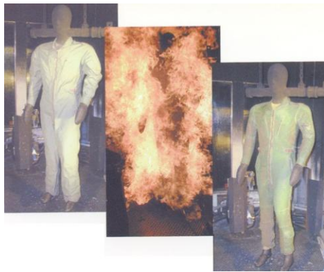
Fig.1 Mannequins dressed with "Nomex" for test in a camera
