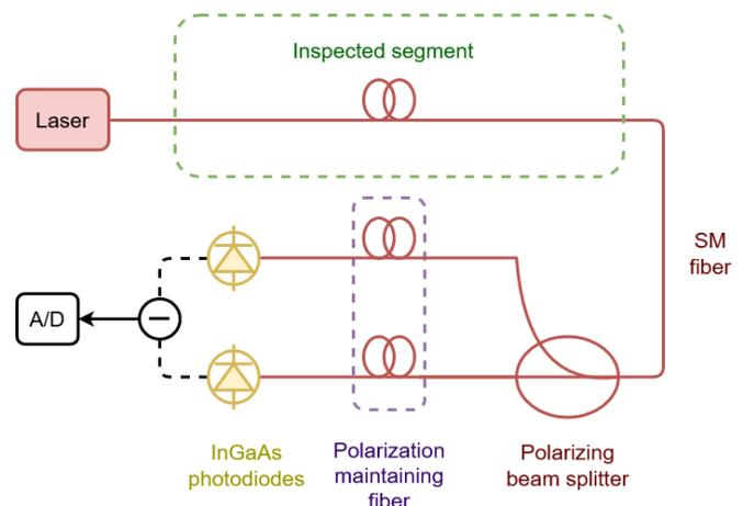
Fig. 1: Scheme of the system for the detection of SOP changes.
