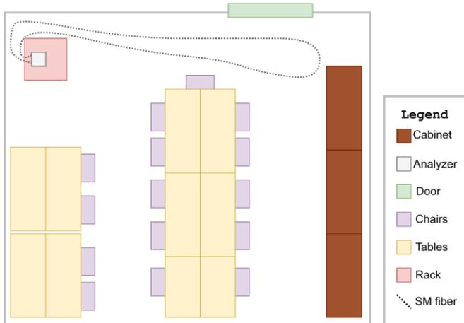
Fig. 4: Scheme of a laboratory for intrusion testing in a server room equipped with analyzers and SM fiber.
