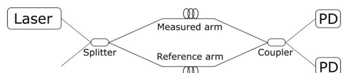
Fig. 2: Schematic of the Mach-Zehnder fiber interferometer [10].
