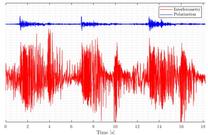
Fig. 5: Comparison of methods. Vibration caused by opening and closing rack doors.
