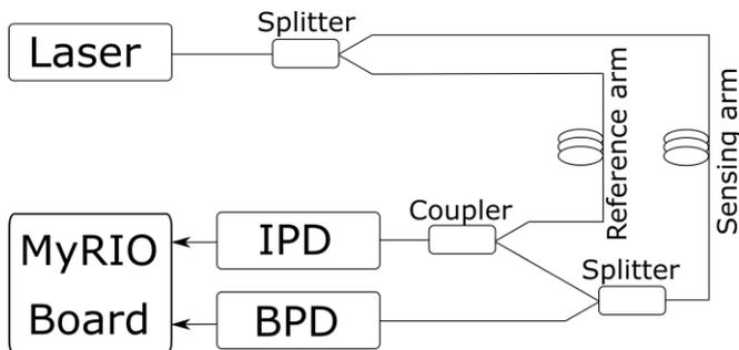
Fig. 3: Scheme evaluation setup with Mach-Zehnder interferometer and SOP analyzer.
