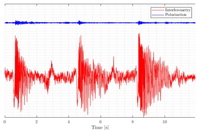
Fig. 6: Comparison of methods. Vibration caused by opening and closing entrance doors.
