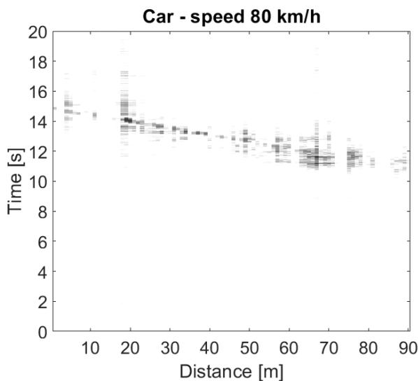
Figure 8 Car by fiber at 80 km/h.
