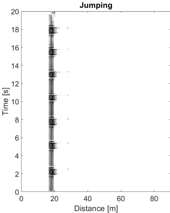
Figure 3 Jumping of person near fiber.
