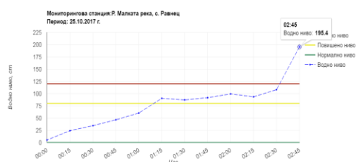
Fig. 7 Water level of Malkata reka river 0.00-2.45 o'clock
