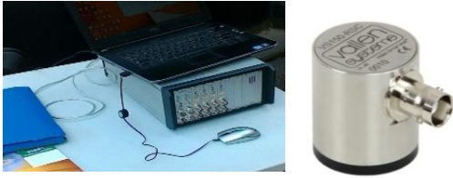
Fig.3.1. Vallen System AE processor unit (below) with the recording PC (on top) AE sensor VS-150-RSC
