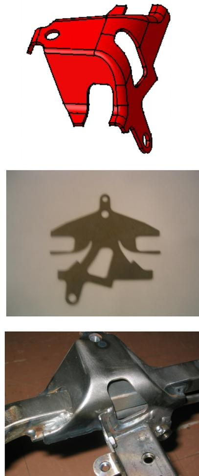
*Fig. 6 Process of prototyping the complex element.*
