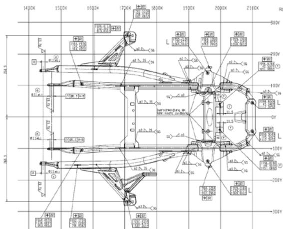
Fig. 2 Drawing of the product rear frame K71.
