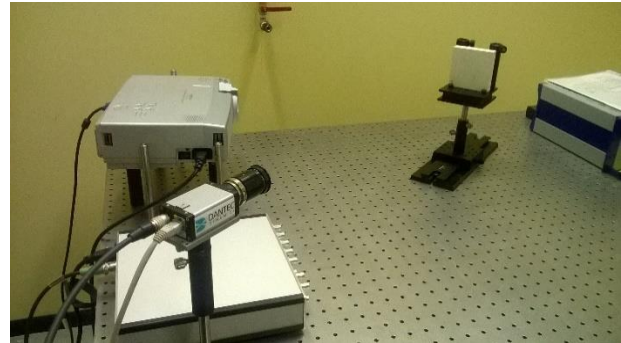
Fig.1 Triangulation scheme of the measuring system
