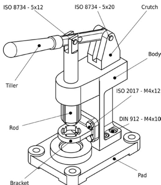
Fig.2 Exemplary assembly “Ring checker”
