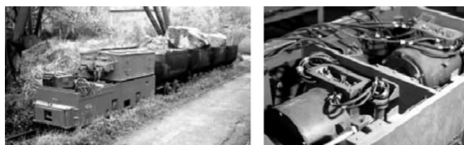
Fig. 2 Common view of the traction locomotive and placement of the electric motors.
