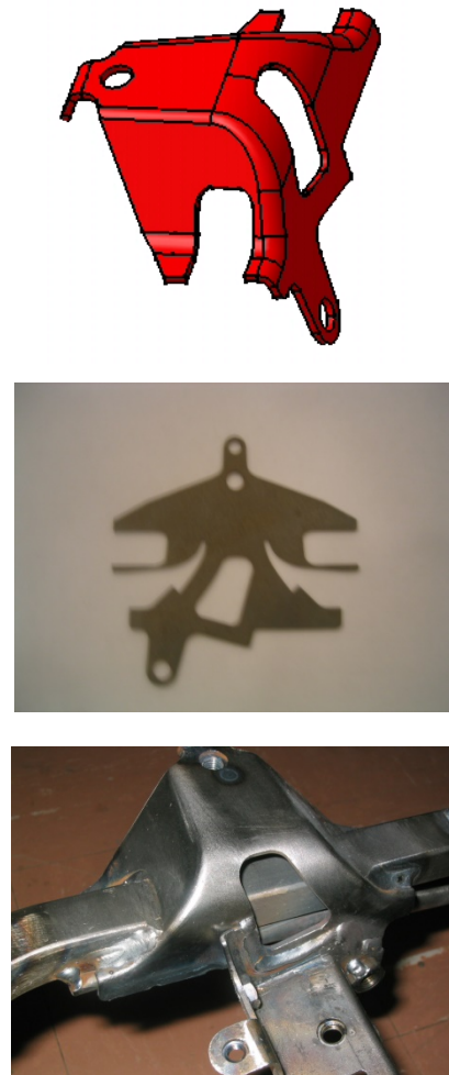
Fig. 6 Process of prototyping the complex element.
