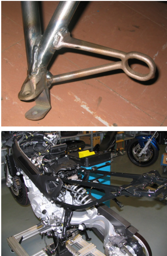
Fig. 5 The exhaust bracket, made with DMLS rapid prototyping technology and its position on the bike.
