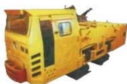
Fig. 1 Contact mine electric locomotive of type 10KR.
