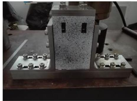
Figure 4. Edge-constraint structure adopted in the experiment
