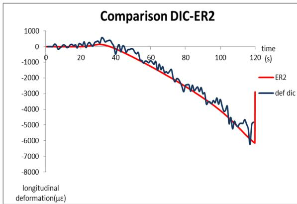
Figure 7. Comparison of longitudinal deformation reading between DIC and strain gauge
