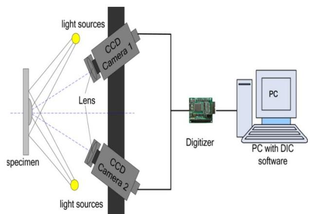
Figure 2. Schematic of a complete 3-D DIC system [6]
