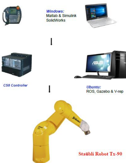
Figure 4: Control Diagram of Stäubli Robot Tx-90
