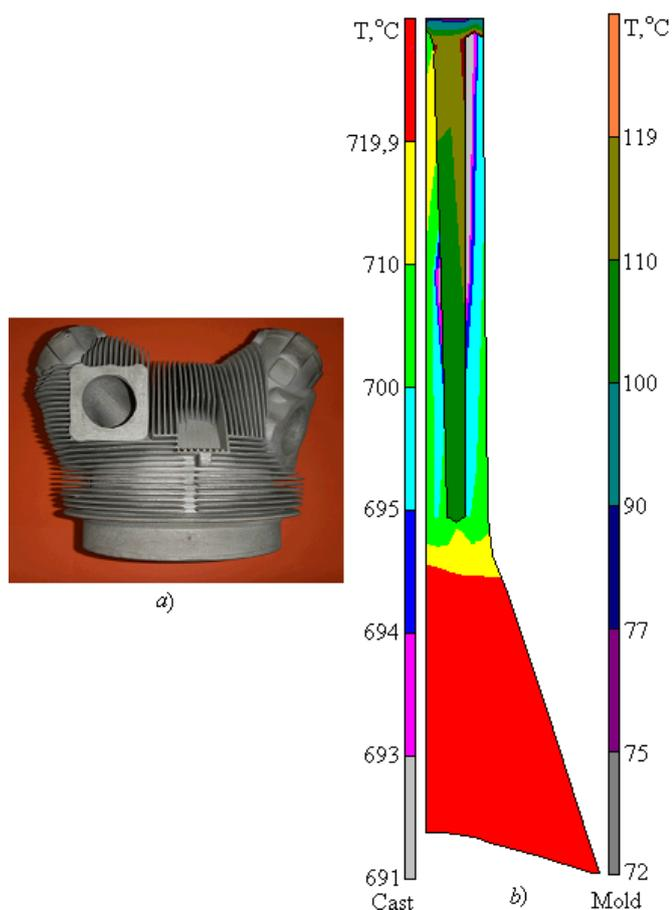
**Fig. 1** The possibilities of die-casting and computational mathematics: a) Cast cylinder head for an aircraft engine produced by the gas counter-pressure process according to [1]; b) Non-stationary temperature field cooling of a local melt volume (rib) and an adjacent local volume of format at the start of a melt cooling process. Computational mathematics allows detailed numerical study of contact heat transfer in volume with complex geometry according to [2]
