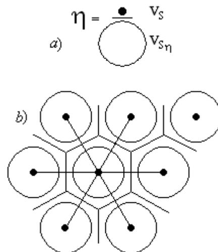
**Fig. 2** Scheme – casting structure of meso- level [3]: a)  $\eta$  – packing density coefficient,  $v_s$  – volume of atom,  $v_{s\eta}$  – volume of cell, where have only one atom; b) 2D an ideal crystal lattice composed of Wigner-Seitz cells.
