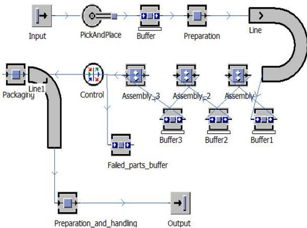
Fig. 4 Base model of system (Tecnomatix Plant Simulate)
