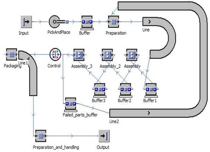
Fig. 5 Adjusted model of the system (Tecnomatix Plant Simulate)
