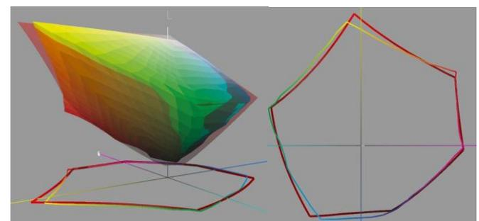
Fig.9 – 3D Comparison of i1Profiler generated profile color gamut and standard offset profile gamut (shown entirely in red)
