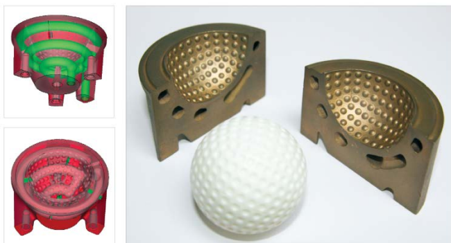
Fig.2.2. Golf Ball blow-mold Left: Conformal cooling Right: Direct Tool cavity (Source: https://www.eos.info )
