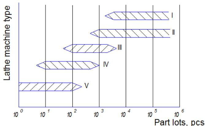
**Fig. 1.** Applications of various lathe machines under a variety of part lots: 1 - drum (rotor) automatic machine; 2 - multiple-spindle automatic machine; 3 - single-spindle automatic lathe; 4 - capstan lathe; 5 - CNC lathe
