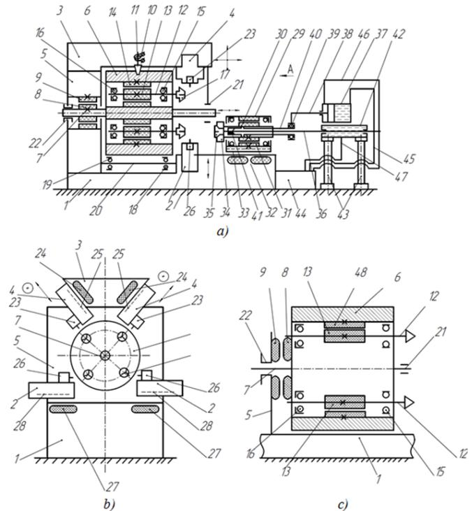
**Fig. 3.** The principal design of multiple-spindle automatic machine: a) spindle drum with a cylindrical-shape motor drive; b) view by arrow A; c) variant of spindle drum with a planar-toroid-shape motor drive
