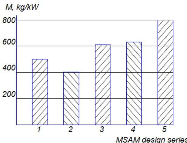
**Fig. 2.** Comparative diagram of metal efficiency in different design series of multiple-spindle automatic machines: 1 – 123; 2 – 1240-6; 3 – Wickman MSAM; 4 – Gildemeister AG MSAM; 5 – KON MSAM
