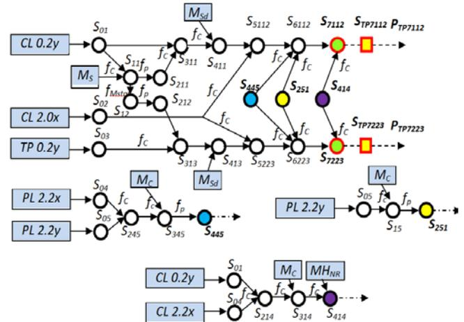
**Fig. 4.** Genetic model of multiple-spindle automatic machine EM-structure synthesis using defined search function  $F_S(2)$ :  $f_c$  – genetic crossing operator;  $S_{01}, S_{02}, \dots, S_{7112}, S_{7223}$  – synthesized structures of electromagnetic chromosomes;  $S_{TP7112}, S_{TP7223}$  – technical solutions;  $P_{7112}, P_{7223}$  – populations of technical solutions
