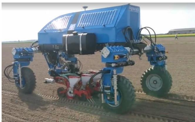
Fig. 2 Robot during sugar beet seeding work
