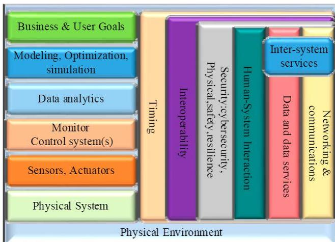
Fig.1: NIST Reference architecture of CPS [14]
