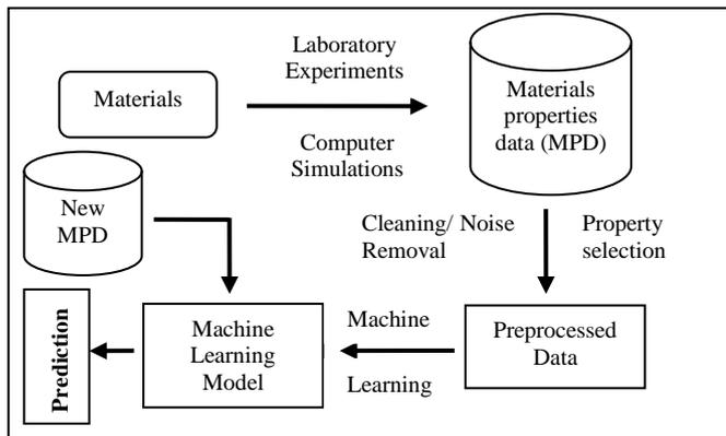
Figure 2: Knowledge Discovery Process using Machine Learning in Material Science
