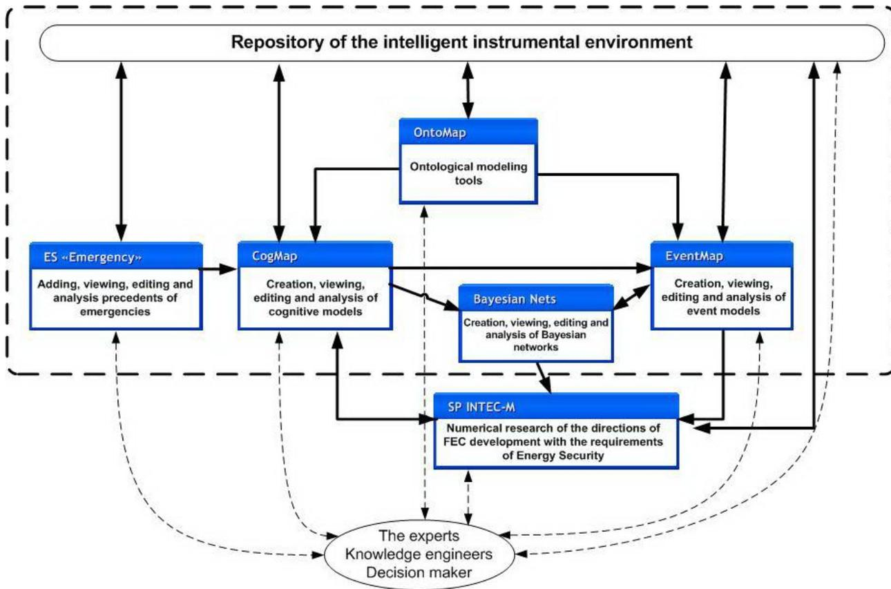
Figure 1 - Interconnection of the tools in the intelligent IT-environment
