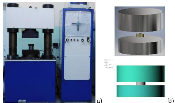
**Fig. 2.** Used Testing Equipment (a) Testing Machine MS-2000; (b) a digital simulation model
