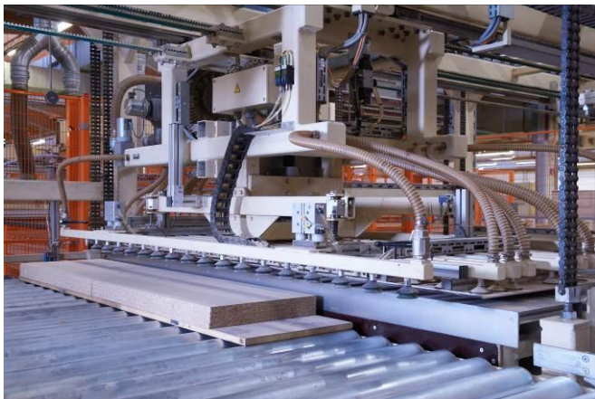
Fig. 2 Automized material handling of a pressing machine
