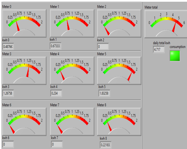
Figure-7: Cumulative consumption meter panel
