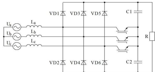
Fig. 5. The scheme of the Vienna rectifier
