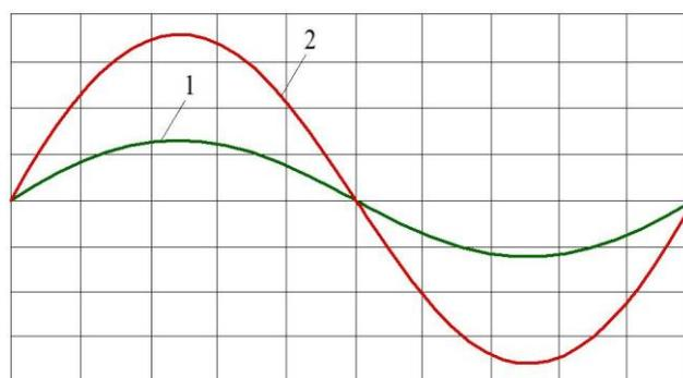
Fig. 2. The diagram of the input current (1) and the voltage (2) of the active step-up rectifier
