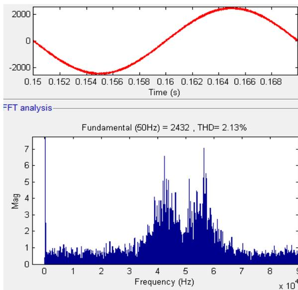
Fig. 10. Fourier analysis of the phase current of the active rectifier
