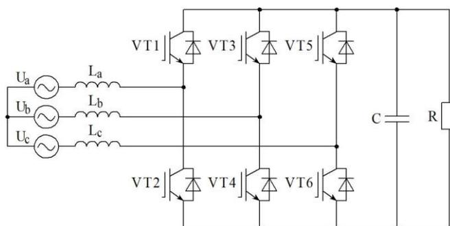
Fig. 1. Two-level active step-up rectifier with correction of power factor
