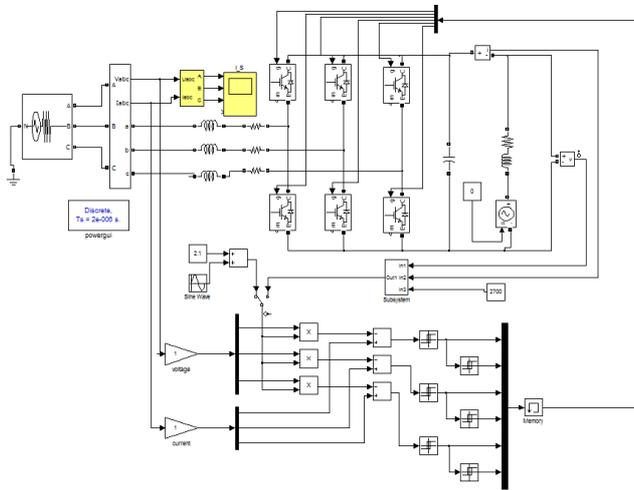
Fig. 8. Imitation model of an active rectifier
