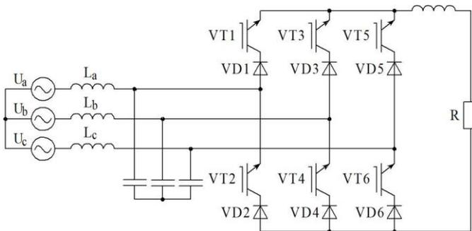
Fig. 4. The active full-wave step-down rectifier
