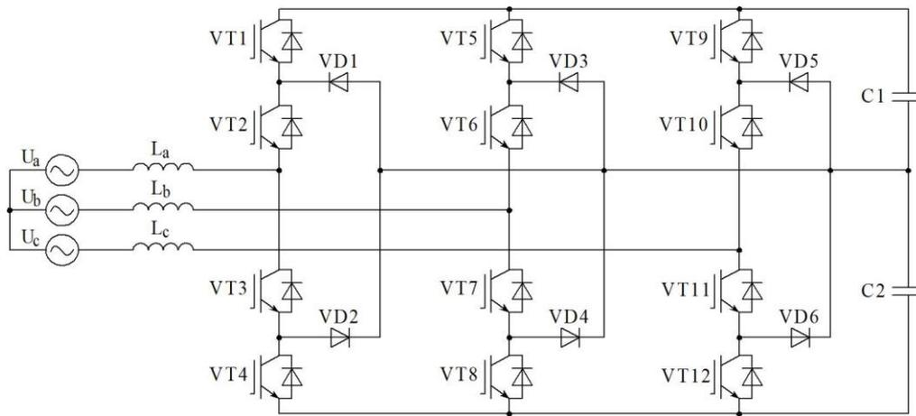
Fig. 3. Three-level active step-up rectifier with correction of power factor
