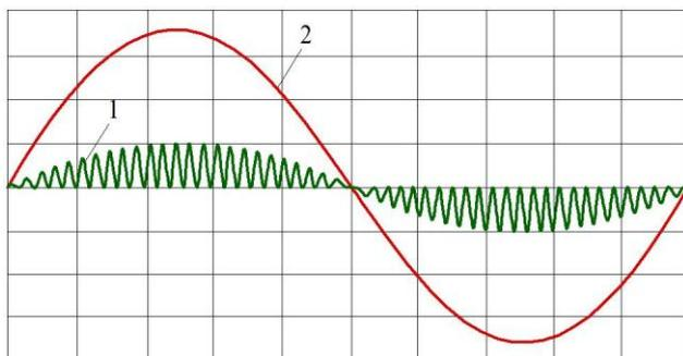
Fig. 7. The input current (1) and the voltage (2) of the single-key step-up converter
