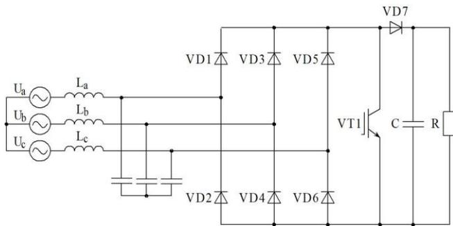
Fig. 6. Single-key scheme of a three-phase active step-up rectifier
