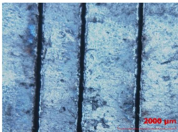
Fig. 5 Photos of the laser cut strips for measuring experiment.
