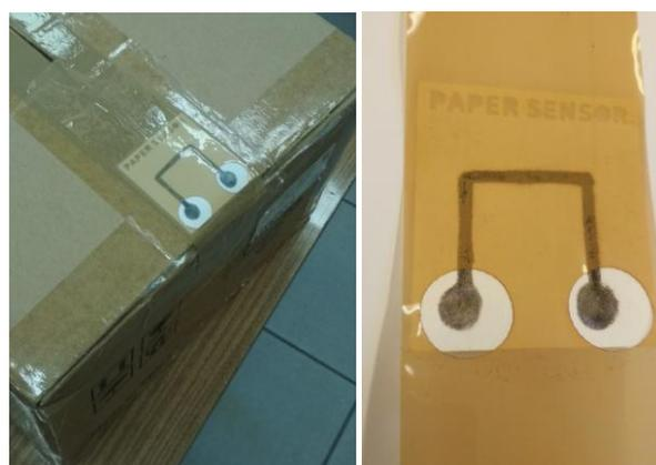
Fig. 6 Photos of the implemented paper sensor with tape.
