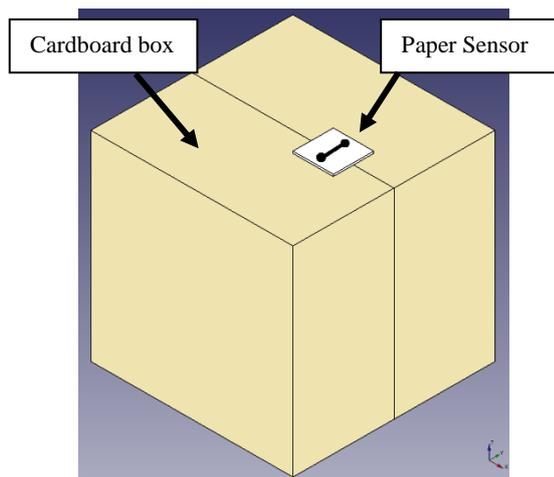
Fig. 1 Visualization of the cardboard box with integrated pencil drawn sensor.
