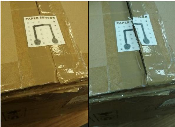
Fig. 7 Photos of the implemented paper sensor (perforated) with glue - closed and opened box.
