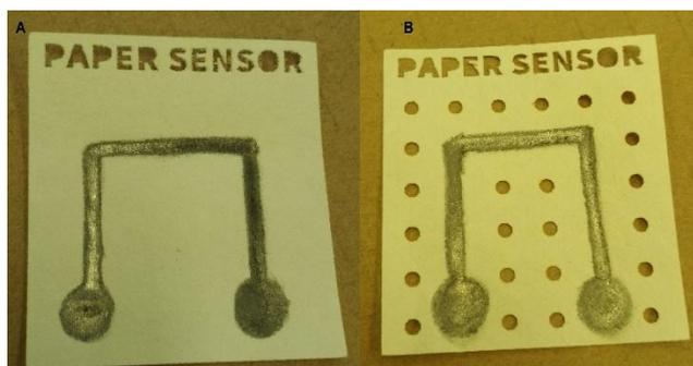
Fig. 4 Photos of the paper sensor -without (A) and with perforation (B).
