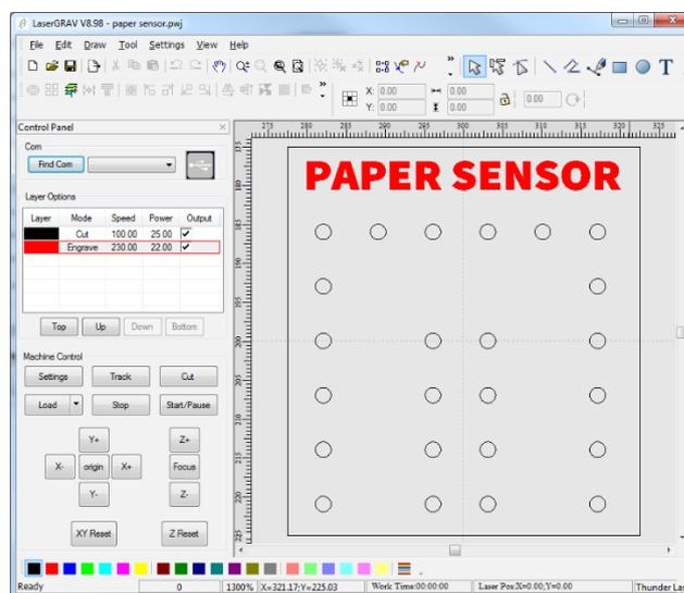
Fig. 2 Screenshot taken from the laserGRAV with sensor's design.
