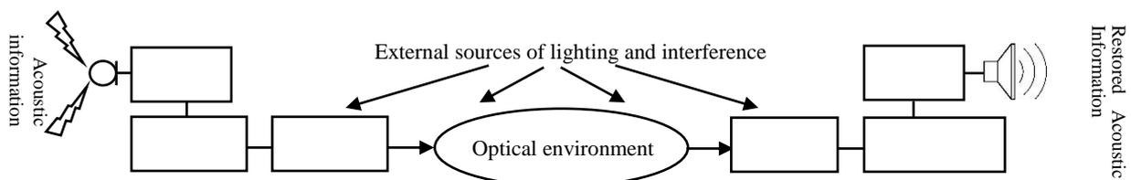
**Fig.1.** Block diagram of the acoustic channel information leakage through the modulation of visible light
