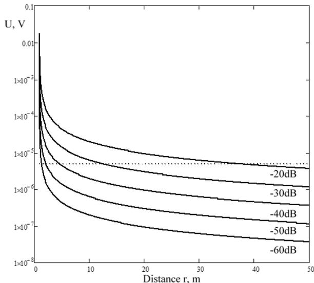
Fig. 2. The dependence of the voltage generated by the sound pressure on the microphone on the distance  $r$  from the speaker with the level  $L_{zv} = 50$  dB. The dotted line corresponds to a level of  $5 \mu\text{V}$ .
