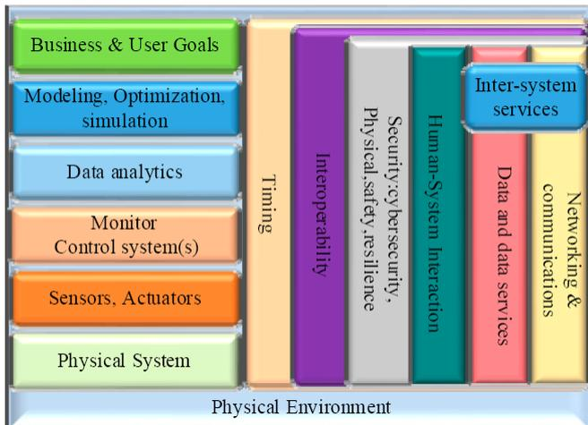
Fig.6: NIST Reference architecture of CPS [13]
