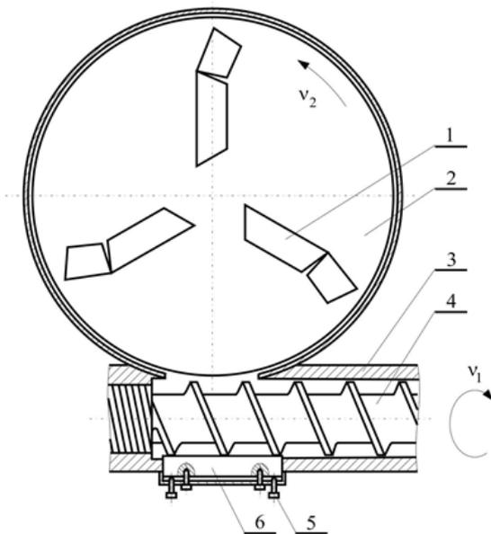
**Fig. 3** Schematic of the longitudinal section of the feed opening and feed sections of an extruder plasticizing system: 1 - sharp working edges, 2 - rotating tool, 3 - barrel, 4 - screw, 5 - adjusting screw bolts, 6 - slat (rib),  $v_1$  - rotational speed of the screw,  $v_2$  - rotational speed of the rotating tool [3]
