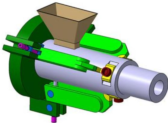
Fig. 11 Concept model No 1. Assembly view
