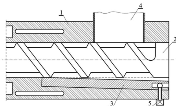
**Fig. 4** Longitudinal section diagram of the adjustable grooved feed section of an extruder: 1 - barrel, 2 - screw, 3 - slat (key), 4 - feed opening, 5 - actuator [4]
