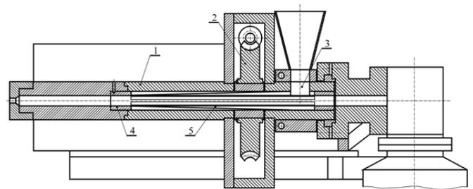
**Fig. 7** Longitudinal section diagram of the active grooved feed section of the extruder which eliminates shifting and deformations of the feed opening: 1 - barrel segment, 2 - worm wheel, 3 - feed opening, 4 - grooved sleeve, 5 - grooves [7]
