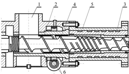
**Fig. 1** Longitudinal section diagram of an adjustable grooved feed section of an extruder: 1 – feed opening, 2 – sleeve with a spiral undercut, 3 – cooling channels, 4 – screw, 5 – barrel, 6 – worm gear [1]
