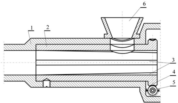
**Fig. 6** Longitudinal section diagram of the active grooved feed section with the twisting sleeve: 1 - barrel, 2 - grooved sleeve, 3 - grooves, 4 - worm wheel, 5 - worm, 6 - hopper [6]
