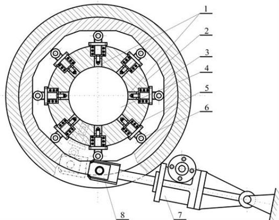
**Fig. 2** Schematic of the cross section of a plasticizing system with an active grooved feed section: 1 - adapters, 2 - rotationally fixed sleeve, 3 - rotatable sleeve, 4 - feed opening, 5 - spring, 6 - roller, 7 - lifting spindle gear, 8 - bolt [2]
