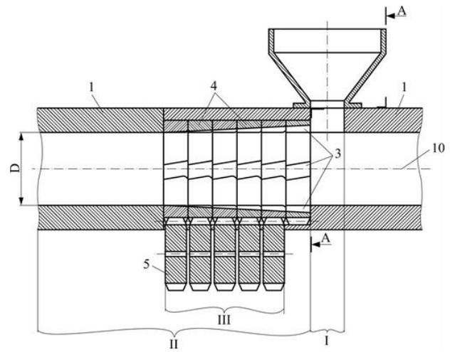
**Fig. 10** Longitudinal section diagram of the active grooved feed section of an extruder with a twistable sleeve formed by rotary ring segments: a) before twisting, b) after twisting; 1 - barrel, 2 - right-handed grooves, 3 - longitudinal grooves, 4 - rotary ring segments, 5 - worm wheel, β - groove twisting angle [10]
