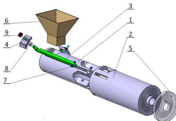
Fig. 14 Concept model No 2. Exploded view: 1 – main sleeve, 2 – barrel, 3 – moving segment, 4 – fixing element, 5 – separating cooling disc, 6 – hopper, 7 – fixing pivot, 8 – adjusting screw, 9 – nut
