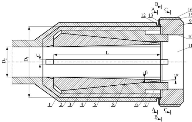
**Fig. 8** Longitudinal section diagram of the active grooved feed section of an extruder equipped with a set of slats and wedges set into motion by a rotary ring: 1 – grooved sleeve, 2 – barrel, 3 – slat, 4 – wedge, 5 – rotary ring, 6 – groove with adjustable depth [8]
