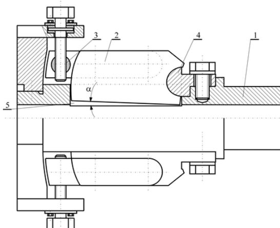
**Fig. 5** Longitudinal section diagram of the active grooved feed section with four longitudinal grooves, description in the text [4]
