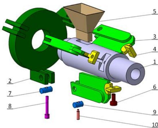
Fig. 12 Concept model No 1. Exploded view: 1 – main sleeve, 2 – fixing plate, 3 – moving segment, 4 – hinge, 5 – hopper, 6 – fixing screw, 7 – front pivot, 8 – adjusting screw, 9 – back pivot, 10 – adjusting metal bolt
