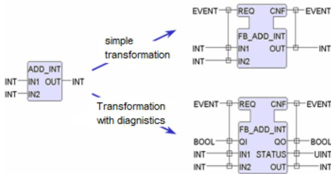
Fig.5: Transformation of PLCopen to IEC 61499 Standard
