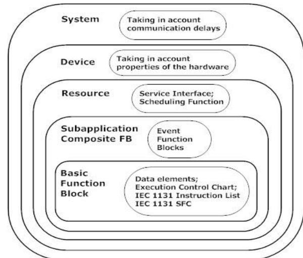
Fig.1: Overview of IEC-61499 based models
