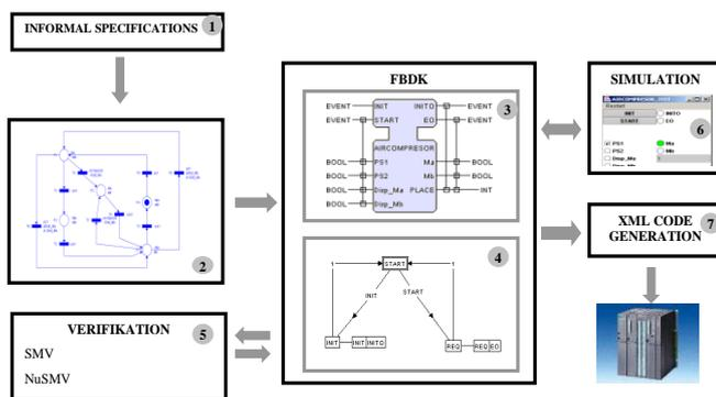
Fig.3: Combined approach using IEC-61499 standard and formal specification
