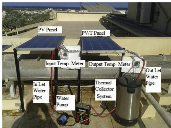
Fig.8. Experimental setup of PV/T system and referent PV panel [18]
