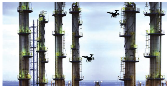
Fig. 7 Drones used for monitoring of industrial safety in USA (image retrieved from [10])
