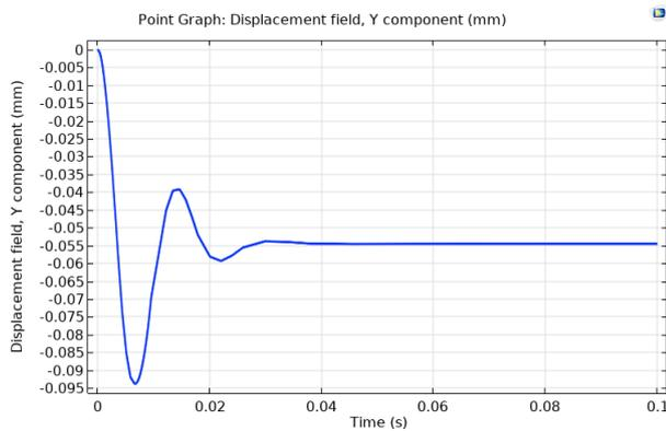
Fig. 6. The proof mass dynamic displacement plot
