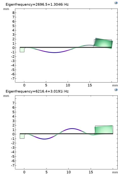
Fig. 8. The third and fourth natural shapes of investigated piezo beam
