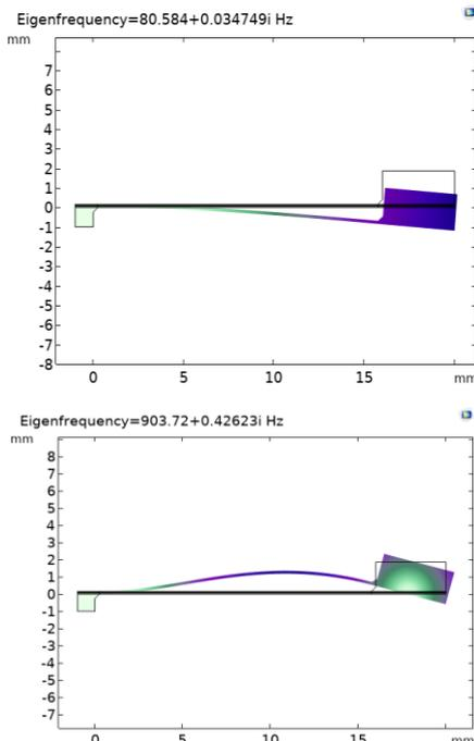
Fig. 7. The first and second natural shapes of investigated piezo beam
