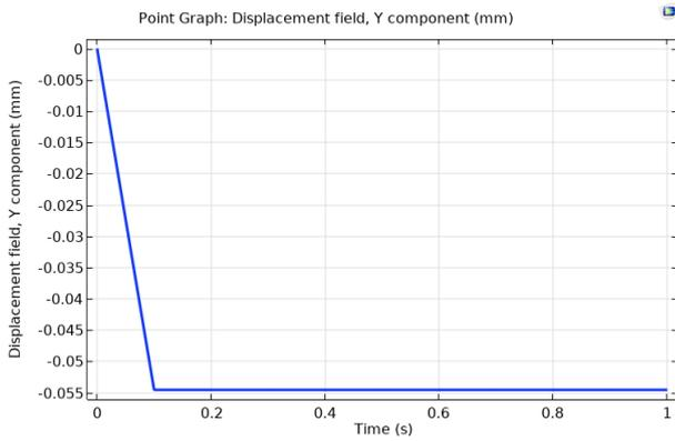
Fig. 5. The proof mass static displacement plot
