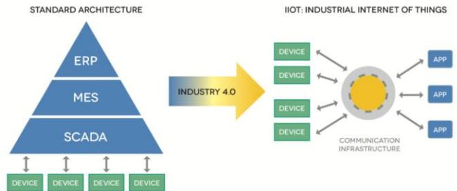
**Fig. 2** The basic Industry 4.0 idea is a change of hierarchical control structure to open communication interface between independent and intelligent objects.
