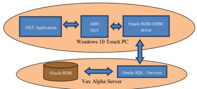
Fig. 2. Schematic representation of the communication between Oracle RDB and client .NET application
