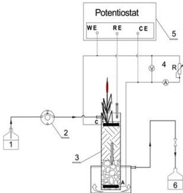
**Fig. 1** Design of Plant sediment microbial fuel cell
