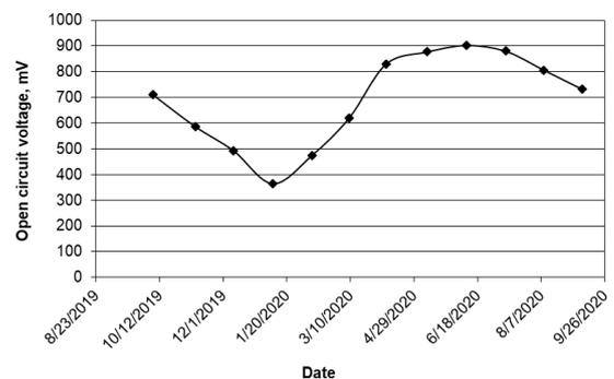
**Fig. 4** Open circuit voltage of PSMFC in different seasons
