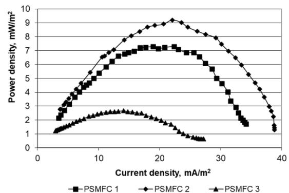
**Fig. 3** Power density of PSMFC-s planted with different vegetations
