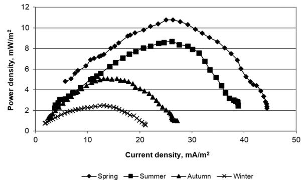
Fig. 8 Polarization curves of PSMFC-s in the four seasons
