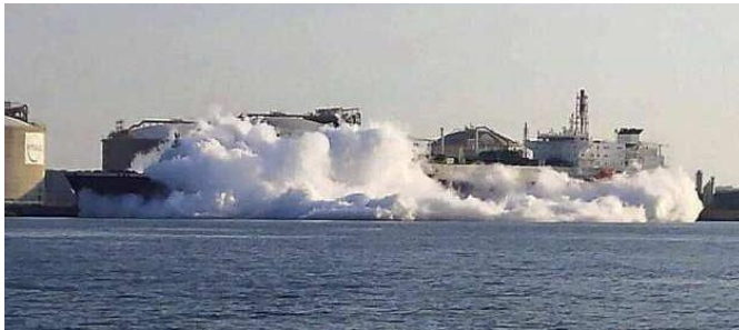
Fig.4 An example of an LNG spill. Source: Hine, L., MOL outlines lessons learned from LNG ship cargo release, 21.07.2016.
