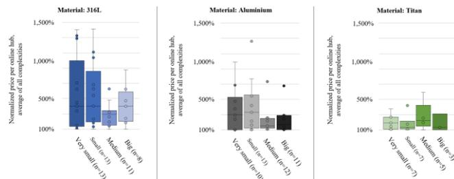
**Fig. 6** Pricing range of online hubs for metal objects with multiple sizes at quantity one.
