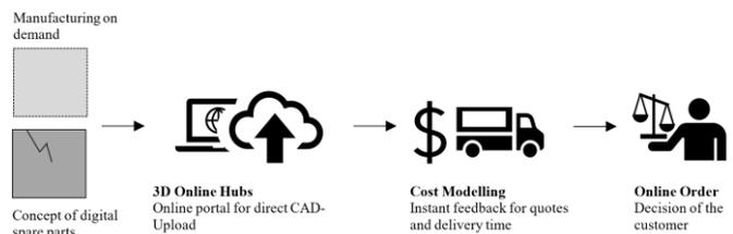
**Fig. 1** Process of Direct Digital Manufacturing via online hubs.
