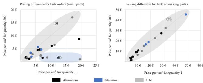
**Fig. 5** Economies of scale for pricing at online hubs (small parts, left; big parts, right).
