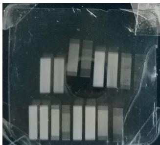
Fig. 5 Image of femtosecond laser patterned thin film of silk fibroin. Creation of modification zones under irradiation with a range of laser parameters.
