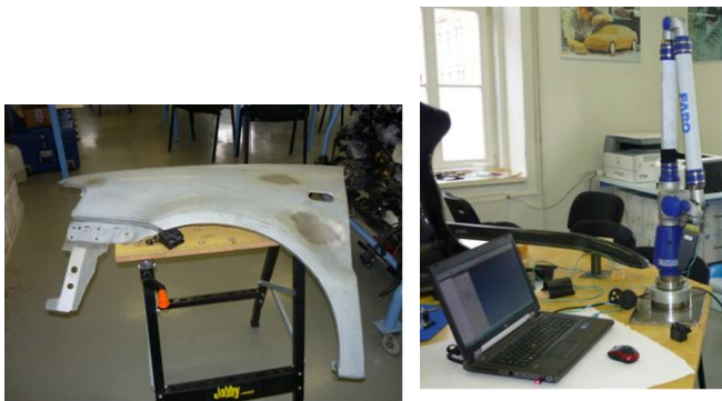
Fig. 1 Front fender of the car and FARO Platinum Arm Laser Scan V3 connected to PC
