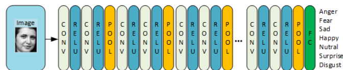
Fig. 3 Typical architecture of CNN for FER
