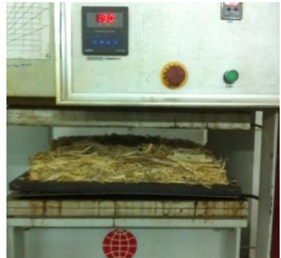
**Figure 3.** Hot pressing of OSB mat.
