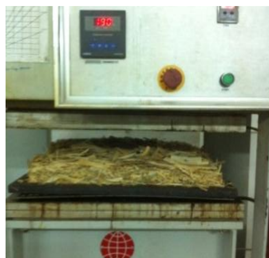
Figure 3. Hot pressing of OSB mat.
