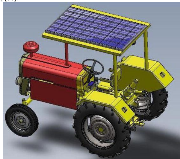
Fig. 8: Schematic diagram of solar powered tractor [36]
