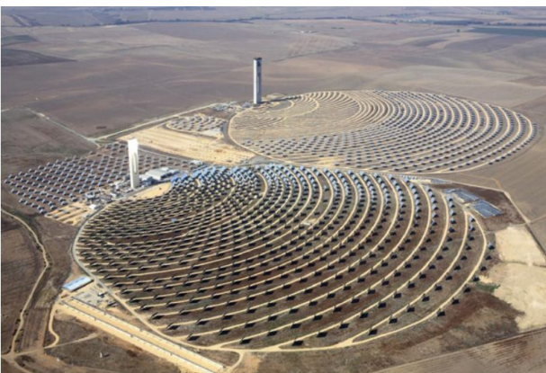
Fig. 4: Solar tower power plants PS10 and PS20 near Seville, in Andalusia (Spain) [20, 26]
