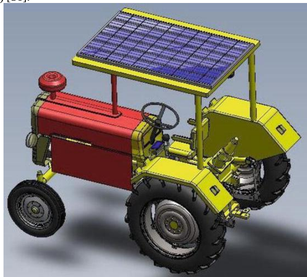
Fig. 8: Schematic diagram of solar powered tractor [36]
