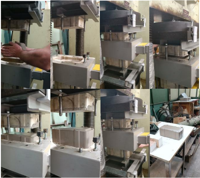
Fig. 7 Plastic molding process with the following steps: loading a plastic mass blank with a weight of 5.100 kg, pressing with a pressure of 13 t/cm 2 , separating the pressed product by pushing it out from the lower punch.
