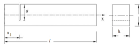
Fig. 1. Specimen with an artificial rectangular channel type crack
