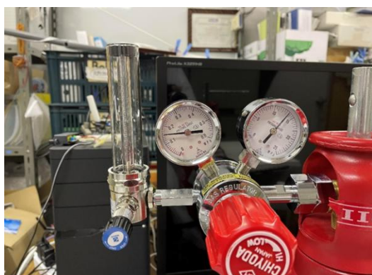
Fig. 3. From the right, a hydrogen cylinder, a pressure regulator, and a flow meter ( H_2 2000cc/min)
