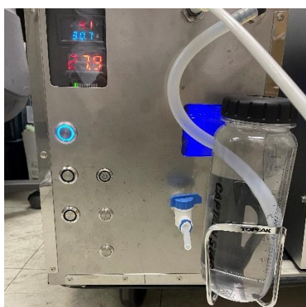
Fig. 4 Oxygen and hydrogen gas generator (TED-CUBE, WAC Inc.) ( O_2 1000 cc/min, H_2 2000 cc/min)
