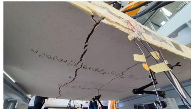
Fig. 10 Tensile failure of the gypsum-fiberboard
