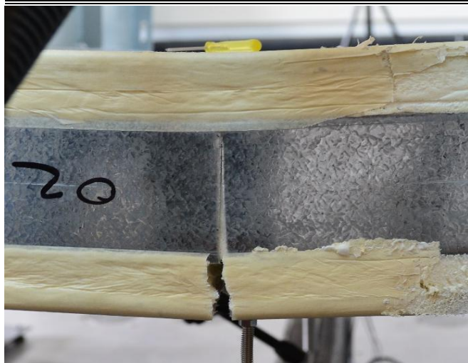
Fig. 12 Tensile failure of one of the outer C-profile
