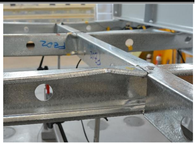
Fig. 9 Failure mechanism in steel core structure specimen
