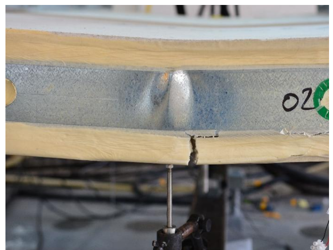
Fig. 11 Failure of the polymer foam
