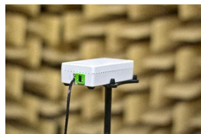
Figure 3. Measurement station positioned within the anechoic chamber.
